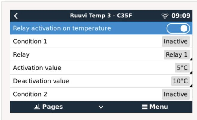
If that is insufficient to maintain the battery temperature above 5 degrees, you may wish to connect a 2nd heat pad contactor to Relay 2 as well.
