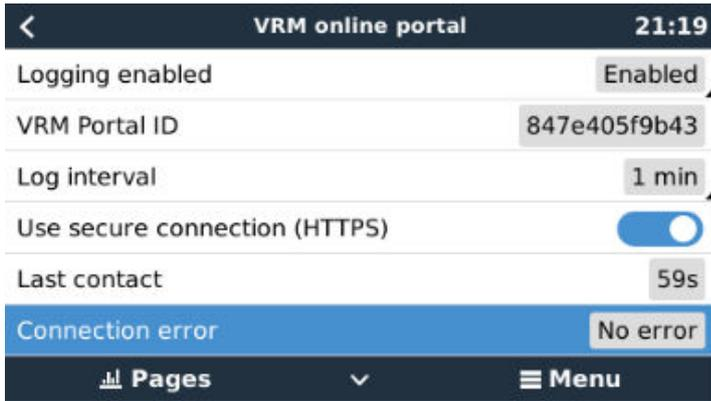
If a Connection error is shown, the VGX is not able to contact the VRM database. The connection error will show an error code that indicates the nature of the connectivity problem. Also, details of the error message are shown, to facilitate on site IT experts to diagnose the problem.
