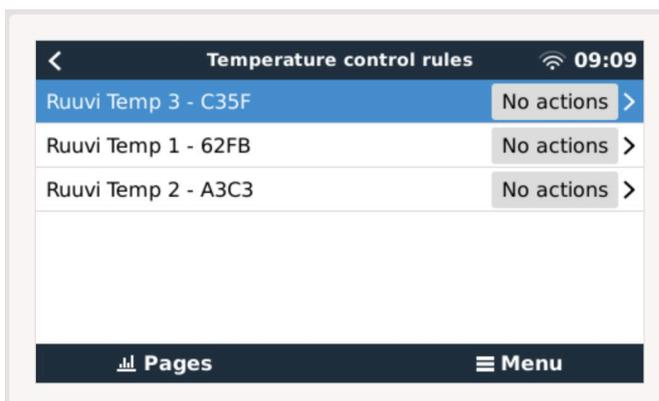
In GX products where two relays are available (Cerbo GX) it is possible to have a single temperature sensor control both relays. It is also possible to have a single relay controlled by multiple different temperature sensors.
