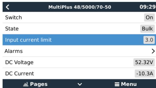
The limit as set by the user in the VGX will be applied to all inputs where 'Overruled by remote', configured with VictronConnect or VEConfigure, is enabled:
