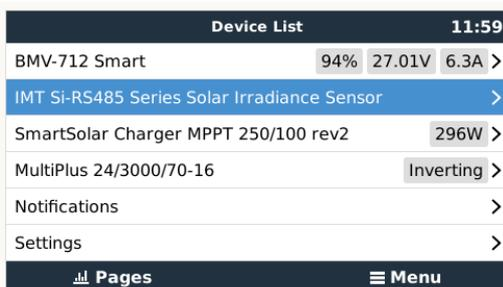
Within the ‘IMT Si-RS485 Series Solar Irradiance Sensor’ menu all available parameters will be automatically displayed (dependent on the sensors connected) and update in real time.
