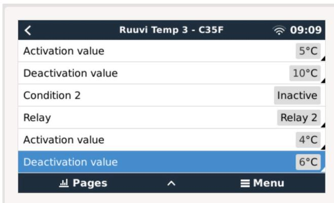
This will mean that Relay 1 will be active if the battery temperature falls to 5 degrees. If the temperature continues to fall below 5 degrees to 4 degrees, then the second heat pad will be engaged via Relay 2.
