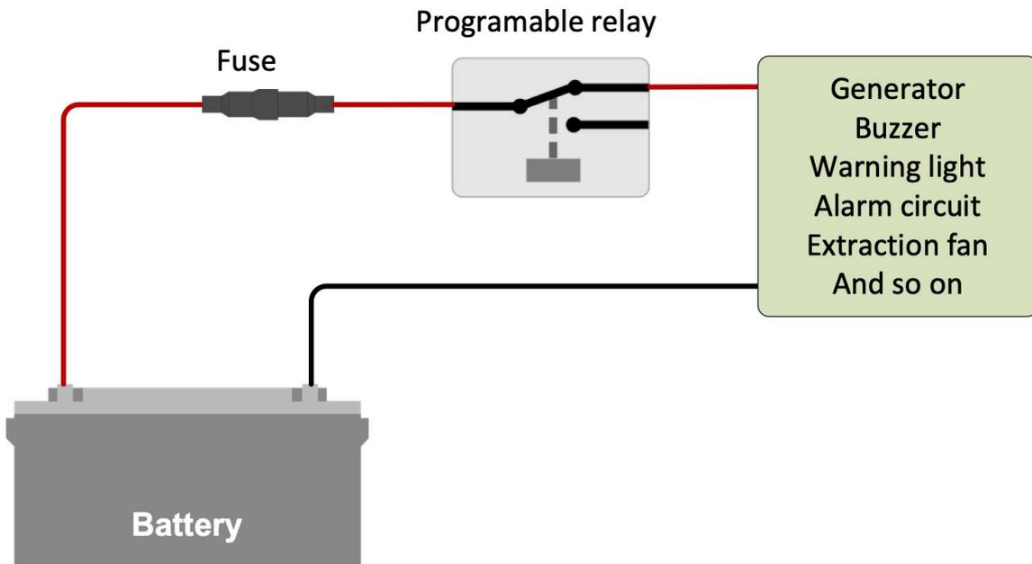
Figure 2. Programmable relay wired to operate as a potential free contact switch
