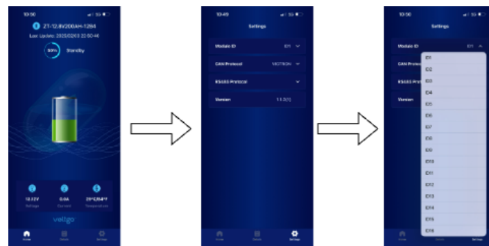
Figure 7. VoltGo battery app to change battery ID number.
