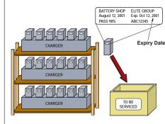
1) Sorting batteries to be serviced. Each time a battery is taken from the charger, the user checks the service date on the attached label. If the date has expired, the battery is placed in a box marked "To be serviced."
