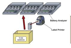
2) Servicing expired batteries. Batteries with expired dates are exercised. Those that fail to recover are reconditioned. Restored batteries are recertified by attaching a new label with dates and capacity reading.
