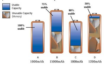
Each of the four batteries show large variations in usable capacity. The larger batteries (B & D ) offer less capacity than the smaller ones (A & C). The weak batteries charge guicker and remain on 'ready' longer than good packs. The weak batteries become a target for the unsuspecting user.
