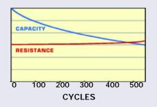
Resistance does not provide a reliable indication on capacity fade that occurs with cycling.  $QuickSort^{TM}$  is based on the electrochemical dynamic response of the battery, a method that is superior to resistance readings.
