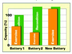
formation or memory. The chart shows capacity doubling with *Recondition* on faded batteries and performance improvement on a new battery.
