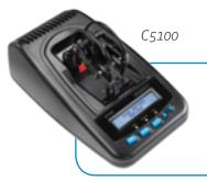
**Mobile Devices** - Batteries are blamed for most cell phone problems. To satisfy the customer, batteries are replaced, often to have the fault recur. The Cadex C5100 battery analyzer assists by performing QUICKSORT™ testing at storefront.
